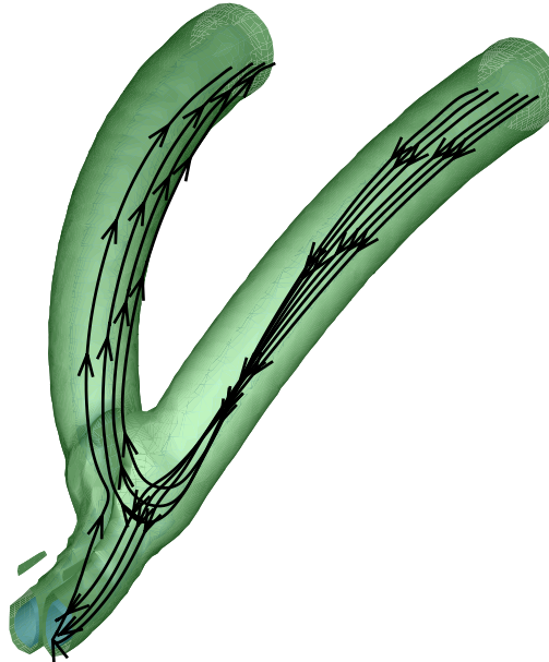
FIGURE 5.14: Cross-over of vortex lines. Vortex tubes shown as iso-surfaces |\underline{\omega}| = 300 \text{ s}^{-1} and 900 \text{ s}^{-1} . Re_{\Gamma} = 1.67 \cdot 10^4 simulation on 128^3 mesh.
