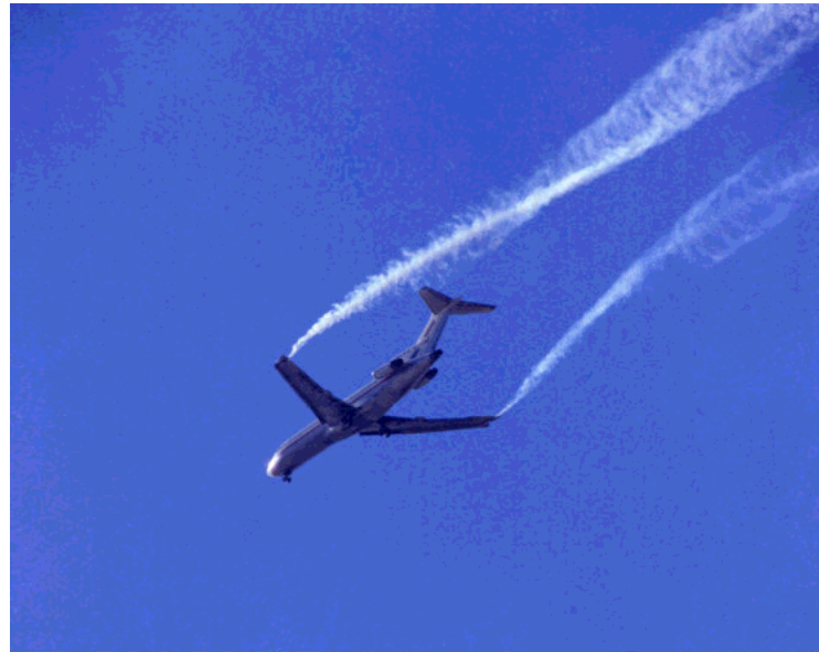
FIGURE 1.2: Visualization (injected smoke) of wing-tip vortex formation: without flap deflection
